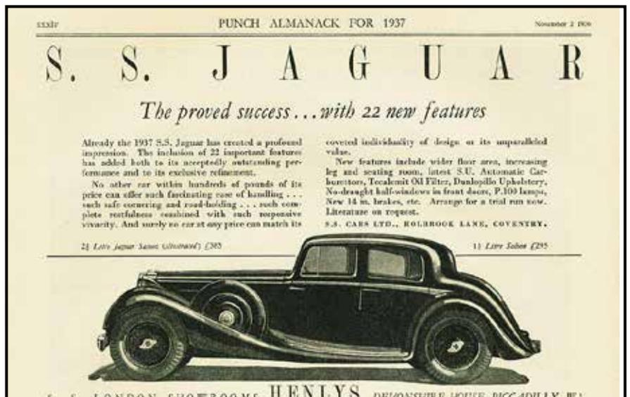
As the builder named it, the "SS Jaguar 2½-Litre Saloon" with its 102 h.p. six cylinder Weslake-designed cross-flow overhead valve cylinder head on its Standard engine caused a sensation when it was launched at a trade lunch
